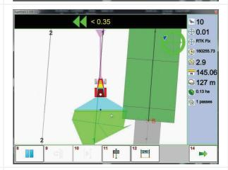
The PAUSE button allows you to temporary stop your work while you have to provide new water to the machine.
