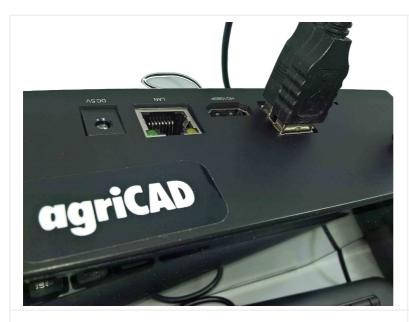
The monitor has 4 USB fitting: two lateral for connecting the Antenna and the system key and two on the top for office use.
