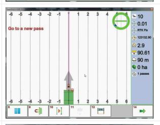
It is possible to quickly set new works thanks to configured data.
